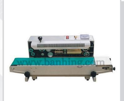
The FR-900 sealer is suitable for small bags packing and adopts electronic constant temperature control system and speed adjusting transmission mechanism. It can seal plastic films of various materials. Such as PE, PP, Aluminum foil. And can be fixed date embossing system. And the newly type(microcomputer control)with counting deice.
