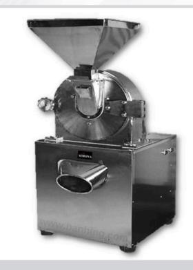
This machine using 204 stainless steel and advanced motor is mainly used in chemical materials, herbal medicines containing
